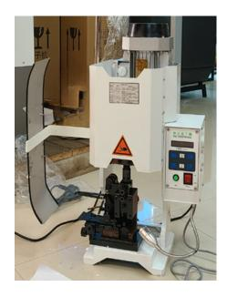
Mute terminal model ultra-quiet terminal machine, using high-tech frequency conversion technology; electronic accurate positioning; motor working noise is smaller than traditional terminal machine when crimping, and power saving; mold adjustment is more convenient and faster; avoid traditional terminal clutch, electromagnet And other common faults!
